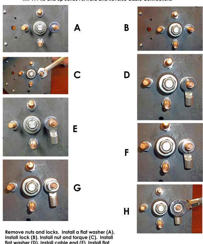
Remove nuts and locks. Install a flat washer (A). Install lock (B). Install nut and torque (C). Install flat washer (D). Install cable end (E). Install flat washer and lock (F). Install nut (G). Torque nut (H).
